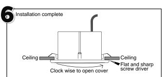
The installation is complete as shown. If is required to uninstall the speaker, use a flat screw driver to pull it down the speakers edge
