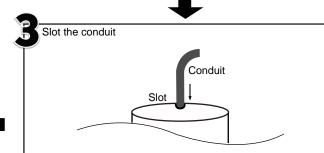
Upon completion of cable termination, the connector can be inserted inside the conduit, and thereafter slot in the conduit into the speaker hole at the back enclosure. The overall installation would look neat.
