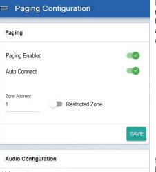
It can be configured to receive or disable paging broadcast, and each speaker assignable with a zone address.
