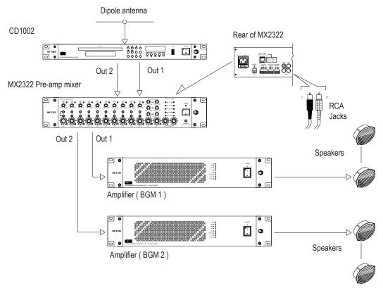
The above schematic shows CD1002 is used to provide 2 sources of BGM to mixer. However, the user shall have the option to :
