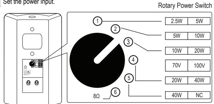
Before install the speaker, adjust the power rating of the unit, to suit the site requirement.
