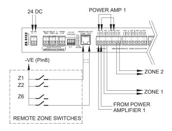
The sample connections shown are using a single unit of either ZS5122 or ZS5062 in a small scale installation. ie. small number of zone outputs.
