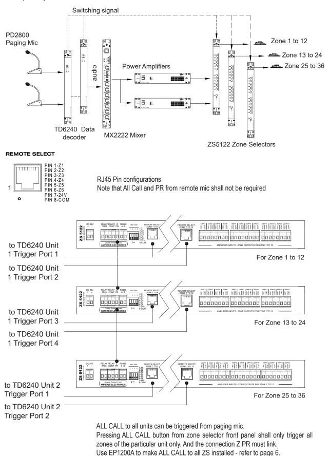
a sample of system with TD6240 zone decoder and few zone selectors
