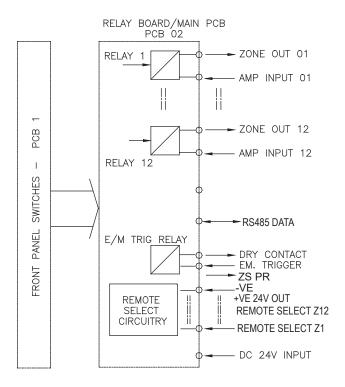
The block diagram shown is for the installer to have a better understanding on how the unit works when interfacing it with other brands of PA equipment.
