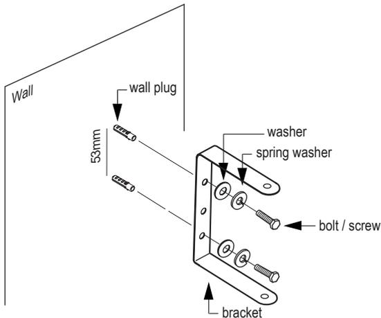
**Note :** Screw / wall plugs for mounting not supplied in the package
