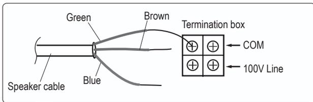
Connect the Green, brown or Blue wire to the terminal box, depend on the desired power ratings.
