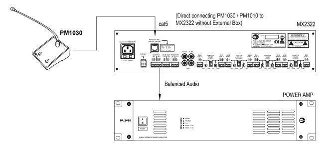
PM1030 can be connected to MX2322 mixer amplifier Remote Mic port without the External Box. With this connection, PM1030 shall has the highest priority over other sources. Take note that with above connection, MX2322 volume control does not amplify / attenuate the mic audio. The mic volume level is fully controlled by the mic volume knob.
