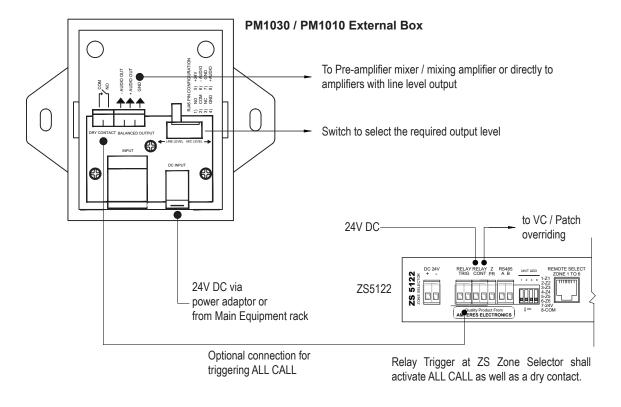
Diagram above shows connection of PM1030 and ZS Zone Selectors ie. External Connector dry contact terminals to Zone Selector's Relay Trigger terminals. Activation of PM1030 shall trigger All Call at zone selector as well as providing 24V DC output to override external volume controllers.
