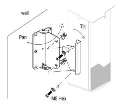
Finally, assemble the completed sub assembly of parts of (2) and (3) with hex screw and nuts provided. The speaker's orientation can be adjusted to pan and tilt. Max pan angle is 170 deg and 30 degree tilt for vertical / horizontal mount.
