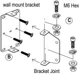
B : Install the wall mount bracket to the wall with self tapping screws provided.
