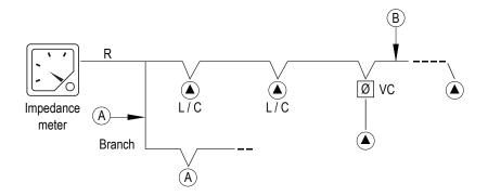
In reality, impedance of a speaker circuit consists of Resistance (normally cable) and Capacitive reactance and Inductive reactance.
