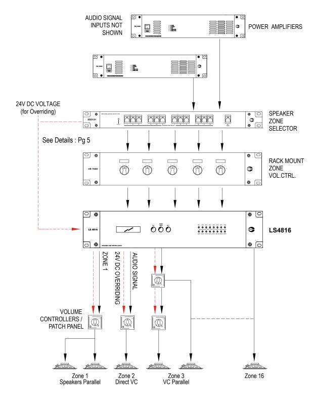
The LS4808 / 4816 detects circuit faults using impedance measurement method. In general, there is no limitation on how the external cabling to speakers or volume controller are run, ie. branching is allow and does not need end line resistors as well as speaker capacitor couplings.
