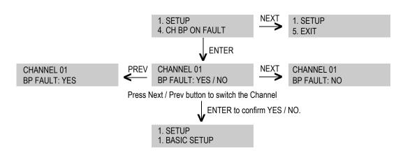
Channel Bypass (BP) can be an option. The user can select the affected faulty channel to be bypassed (on isolated) from connection to the amplifier output. This is to protect the amplifier and also not to interfere with other good zone(s) which are sharing the same power pack.
