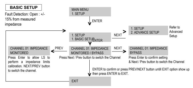
Note: The unit shall measure the impedance of each channel, creating the high and low limits automatically. Whenever the measured impedance falls outside the limits, the channel shall be considered faulty. The limits are typically 15%, eg if the circuit has impedance of 1K  $\Omega$ , the limits generated shall be 850 to 1.15K  $\Omega$ .
