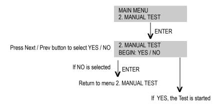
Use this function to test speaker line impedance of each channel.
