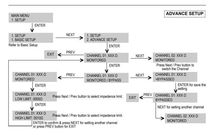
Note: In long cable circuit or zone with multiple branchings the basic mode may not be suitable to detect the fault such as short at the far end of cable (e.g. 500m), cables itself has resistance, thereby would not show short phenomena. It is therefore, Advance setup shall be used.
