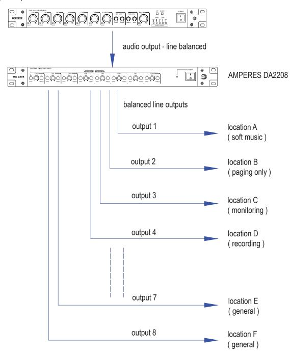
The schematic above illustrates a setup where a single source is to be distributed to different locations (eg. different block of building), and each requires different level of treble or bass.
