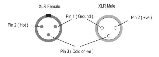
All inputs and outputs available in DA2208 are in balanced mode. In the event that unbalanced signal is to be used, pin 1 and pin 3 shall be shorted.
