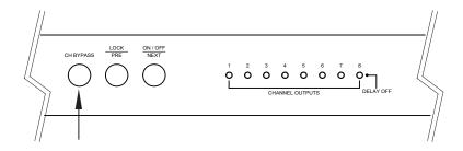
Output channel can be bypassed if required. Follow the sequence below:-
