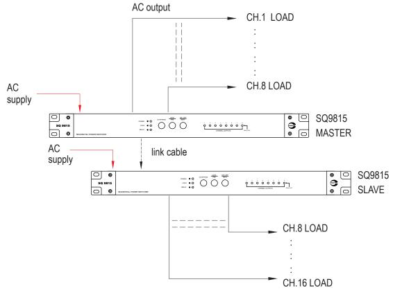
Units shown in cascade mode with 16 channels in total.
