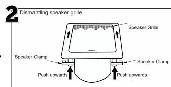
Dismantle the speaker grilles from the speaker assembly by pushing the speaker clamp upwards gently to avoid denting the grille.
