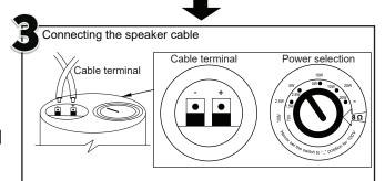
Connect the speaker cable from the ceiling to the connectors provided. Ensure polarity of cable is correctly terminated to the terminals. Pre-select the power output required to suit the installation area before mounting the speaker to the ceiling.
