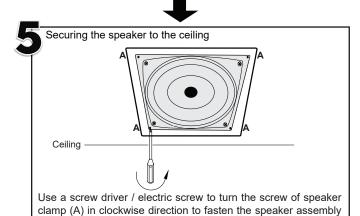
to the ceiling. Ensure a tight clamping for a secure fitting.
