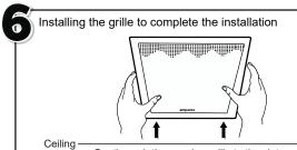
Gently push the speaker grille to the slot without denting the wire mesh.
