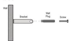
Recommended size for wall screw: Diameter Length 1) Screw M5
