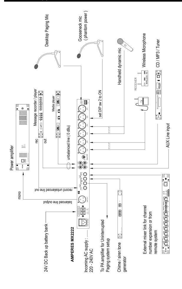
Above diagram shows typical equipments that can be connected to the mixer. Channel allocation for equipment shall not be necessary follow the above illustration.
