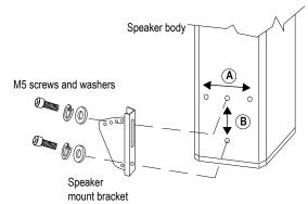
The speaker can be installed in vertical or horizontal orientation, depending on site condition and audio dispersion requirement.
