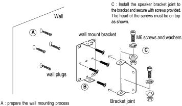
for wall mount bracket. It can be installed horizontally or vertically. Please refer to mounting template.
