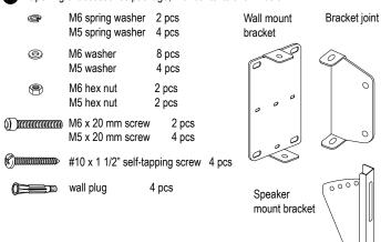
2 Speaker wall mount bracket and bracket joint installation
