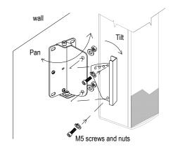
Finally, assemble the completed sub assembly of parts of (2) and (3) with the screws and nuts provided. The speaker's orientation can be adjusted to pan and tilt. Max pan angle is 170 deg and 30 degree tilt for vertical / horizontal mount.
