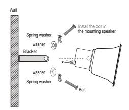
With the bracket securely installed to the wall, mount the horn speaker to the speaker bracket with the screw provided.
