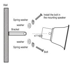
With the bracket securely installed to the wall, mount the horn speaker to the speaker bracket with the screw provided.
